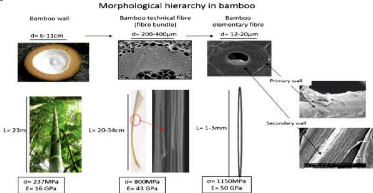
Figure-4. Morphological hierarchy in bamboo[8]
